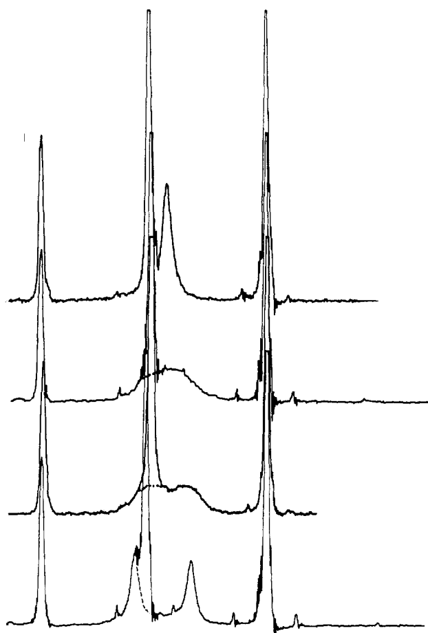
Fig. 2.—Temperature dependence of the gem -dimethyl resonance of 2- t -butyl-3,7,7-trimethylcycloheptatriene (in carbon disulfide with tetramethylsilane as internal standard). The peak at the right is due to the TMS, that at the left to the 3-methyl and the temperature-independent peak in the center is the t -butyl. Reading from top to bottom, the temperatures are -77^{\circ} , -86^{\circ} , -89^{\circ} and -96^{\circ} , respectively. The dotted portions have been added to show the probable appearance of the gem -dimethyl absorption where it is partially obscured by the t -butyl absorption.
